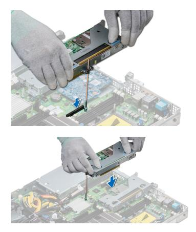
After installing the expansion card riser you could do the following:
