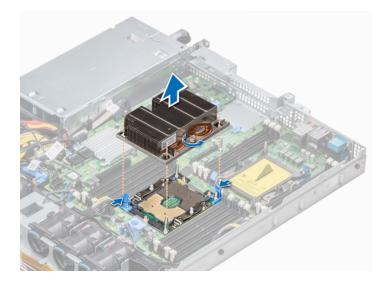
Installing a Processor and Heat Sink Module
