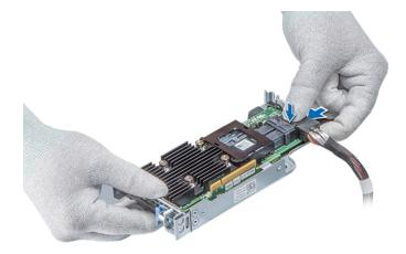
2. Holding the blue touch points, align the slot on the internal PERC riser to the guide on the system board.
