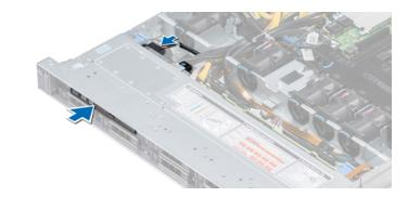
3. Connect the power and data cables to the connector on the optical drive.
