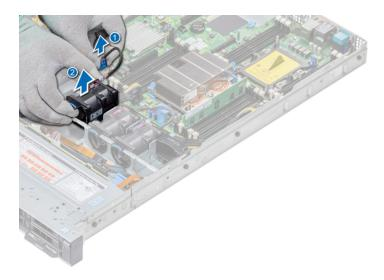
2. Lift the fan out holding the blue touch point.
