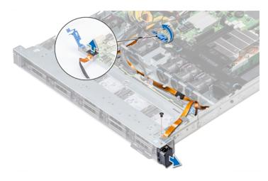
4. Holding the control panel by its sides, remove the control panel away from the system.
