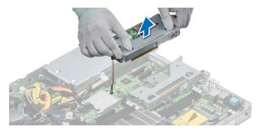
Removing the Expansion card from the Expansion Card Riser
