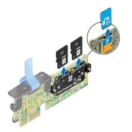
**Note:** Temporarily label each MicroSD card with its corresponding slot number after removal.
