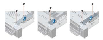
3. Using a Phillips #1 screwdriver, remove the screw that secures the control panel to the system.
