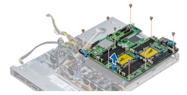
Installing the System Board
