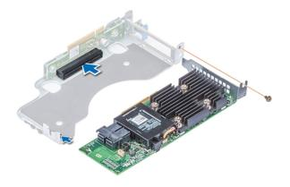
After installing the PERC card from the Internal PERC Riser you could do the following:
