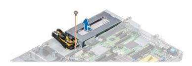
Installing a non-redundant cabled AC power supply unit
