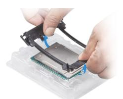
Installing the Processor into a Processor and Heat Sink Module
