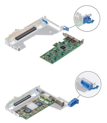
3. Install a filler bracket if you are not replacing the expansion card.
