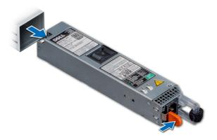
Installing a Power Supply Unit
