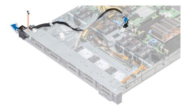
4. Holding by the sides, remove the left control panel assembly away from the system.
