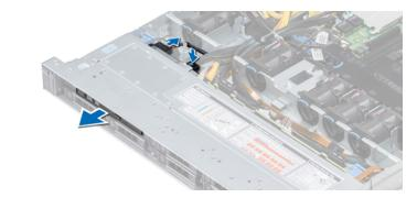
Installing the optical drive
