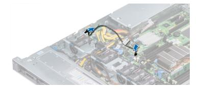
Installing the intrusion switch
